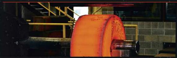
Forging changes the size and shape, but not the volume, of a part. The change is made by force applied to the material so that it stretches beyond the yield point. The yield point is reached when the material will reform into a new shape. Anderson Shumaker has the expertise to form most materials to their required mechanical properties. Shapes include, Rings, Discs, Blocks, Round Bars, Square Bars, Flat Bars and special shapes.
